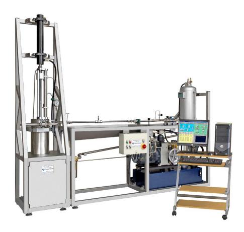
The **TriFlow** TF Series Displacer Primary Liquid Flowmeter Calibration System is the ideal solution for applications where the highly accurate flowmeter calibration is required. It offers a combination of high performance, efficiency and convenience.
