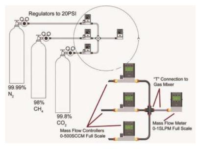
Each MFC has been set to the appropriate pure gas calibration using the gas select screen. The MFCs are receiving their fluctuating flow control ratios by the PC. The MFM is set for N2 as a calibration reference point.
