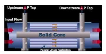
Flow of gas through a Laminar Flow Element generates a pressure difference between the upstream and the downstream pressure tap locations as shown in the cut-away view. This differential pressure is proportional to the flow velocity and viscosity of the gas, according to the Hagen-Poiseuille law.
