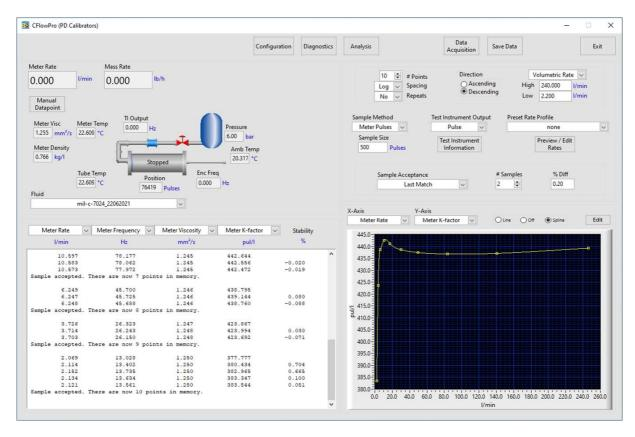
In the process mimic (upper left), the values of all critical parameters can be viewed at a glance. The calibration settings (upper right) configure the software to automatically select and record the desired flowrates in any sequence. As data are collected, they can be observed in real time in numerical as well as graphical forms (bottom).
